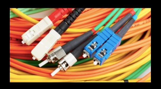
It is the use of thin flexible fibers of glass or other transparent solids to transmit light signals, chiefly for telecommunications or for internal examination of the body. It can transmit data and voice at a longer distance with higher bandwidth. This type of technology provides services such as ethernet, internet, cable tv, and/or telephony services.
